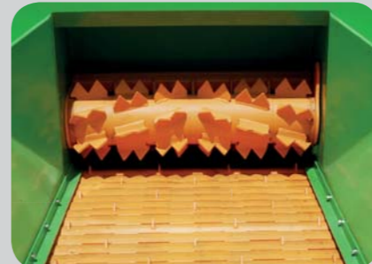
Robust infeed floor with low wear. Infeed opening up to 30cm!
