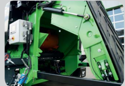
quick and easy exchange of hammers and milling strips
