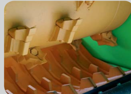
Rotor with fixed hammers and adjustable counterbar
